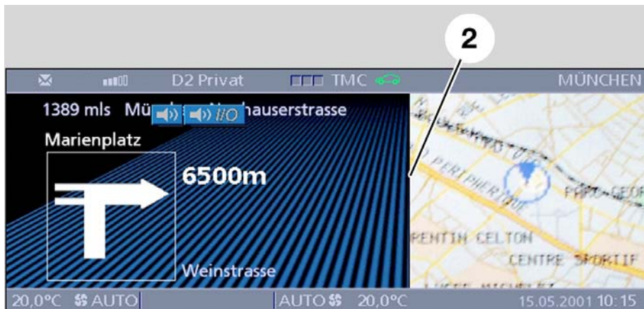
2. Arrow display in control area and map in assistance screen of control display
